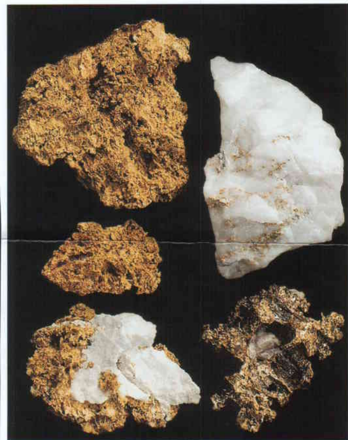
Hand held slot mining produces this specimen stone, which can grade up to 10% gold. Specialists are paid around $100,000 a year, rather than piecework, to ensure maximum safety. Four-six headings are mined at any one time, with serendipity determining which are profitable at over 15g/t and which lose money at under 8g/t. Average grade of this mining over the past six years is 15g/t.
